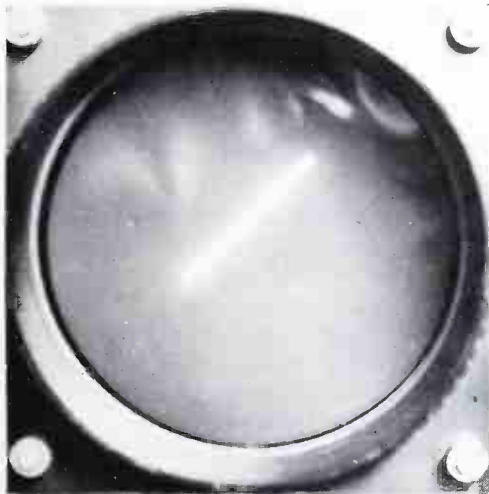
Fig. 3 Another typical out-of-phase trace is shown here, with at least two of the three oscillator signals far off coincidence in the two channels.
