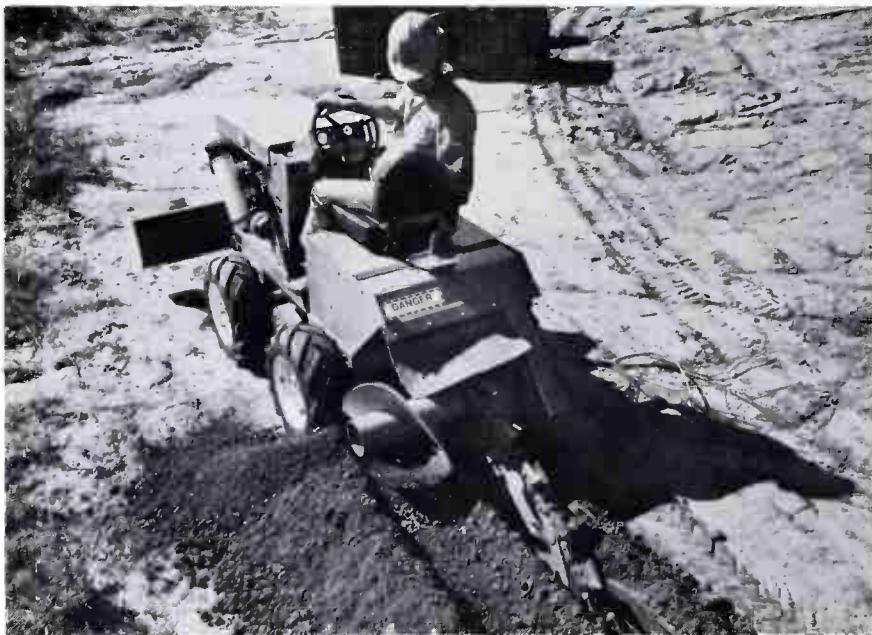
18-HP Model J20 — 4 wheel drive, with three speed forward plus reverse transmission
