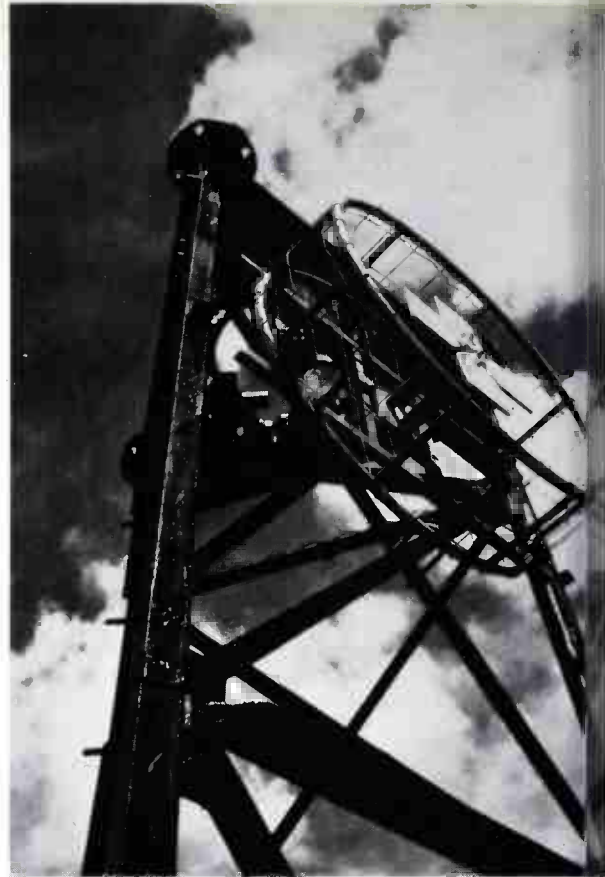
Harris CP antenna has crossed dipoles backed by a cylindrical cavity formed of open wire to reduce wind loading. Rotating field from dipoles excites cavity, which in projection of CP signal at high efficiency.
